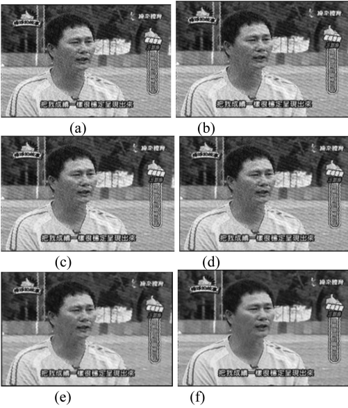
Figure 5. Shows (a) Original Sampling Image; (b) Standard Median Filter [2]; (c) Non-linear Filter [3]; (d) \alpha -trimmed Mean Filter [4]; (e) STS-DDWA Filter [5]; (f) Proposed.
