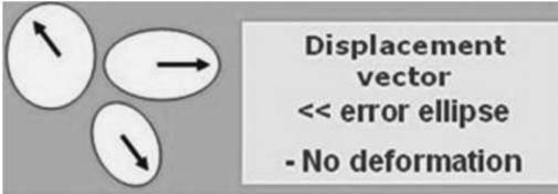
Figure 2. Deformation is not significant.
